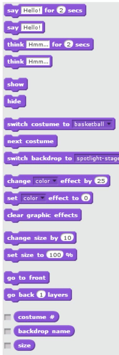
These commands are used to change the appearance of sprites on the stage area. You can make a sprite disappear (**hide**) and reappear (**unhide**). You can also give sprites speech and thought bubbles. You can switch between the various versions (costumes) of a sprite, if you have created them. You can change the size of a sprite and bring it to the foreground if it is positioned behind another sprite.
