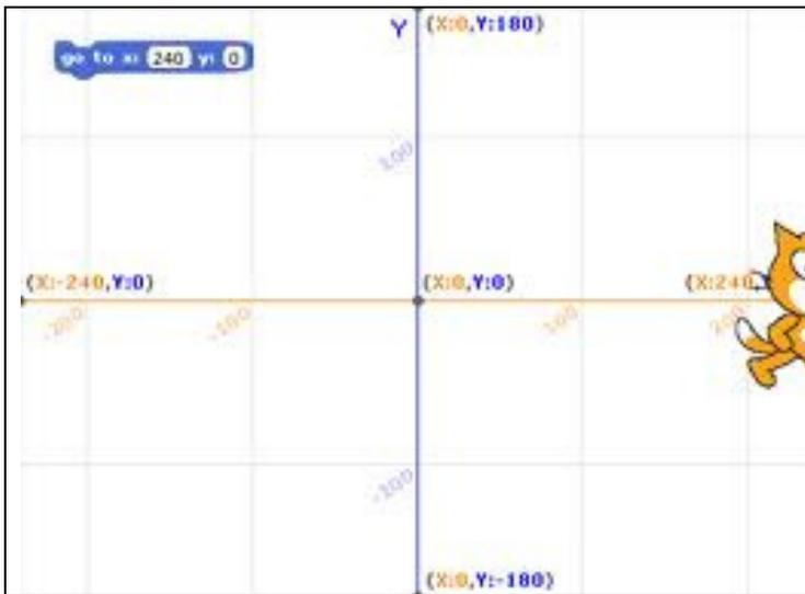
The STAGE therefore has a width of 480 pixels and a height on 360 pixels.
